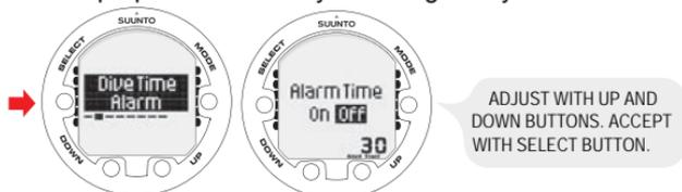
**NOTE** *With a range of 1 - 999 minutes, the alarm can be set to your planned bottom time, for example.*
