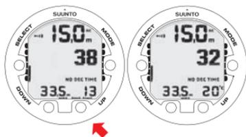
UP BUTTON TOGGLES BETWEEN DIVE TIME AND WATER TEMPERATURE.
