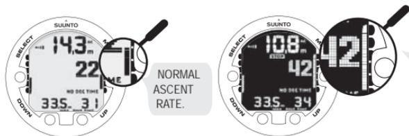
ACTIVATED BACKLIGHT, ALARM AND A BLINKING ASCENT RATE BAR GRAPH INDICATE YOU ARE ASCENDING FASTER THAN 10 M/MIN. YOU ARE ADVISED TO MAKE A MANDATORY SAFETY STOP WHEN YOU REACH A DEPTH OF 6 M.
