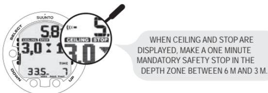
You must not ascend shallower than 3 m/10 ft with the Mandatory Safety Stop warning on. If you ascend above the Mandatory Safety Stop ceiling, a downward pointing arrow will appear and a continuous beeping starts. You should immediately descend to, or below, the Mandatory Safety Stop ceiling depth. If you correct this situation at any time during the dive, there are no effects on the decompression calculations for future dives.
