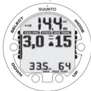
UPWARD POINTING ARROW, BLINKING ASC TIME AND AN ALARM TELL YOU TO ASCEND. MINIMUM TOTAL ASCENT TIME INCLUDING MANDATORY SAFETY STOP IS 15 MINUTES. CEILING IS AT 3 M.
