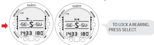
The Suunto Vyper2 also provides help for navigating square and triangular patterns, as well as navigating a return heading. This is made possible by following graphical symbols in the center of the compass display:
