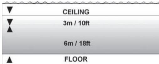
The depth of the ceiling and floor will depend on your dive profile. The ceiling depth will be fairly shallow when you enter the decompression mode, but if you remain at depth, it will move downward and the ascent time will increase. Likewise, the floor and ceiling may change upwards while you are decompressing.
