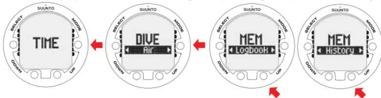
The dive time and date are registered in the Logbook memory. Always check before diving that the time and date are correctly set, especially after traveling between different time zones.
