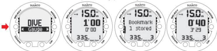
BY PRESSING THE SELECT BUTTON DURING A DIVE, A BOOKMARK IS WRITTEN IN THE PROFILE MEMORY, THE DIVE TIMER IS RESET, AND THE PREVIOUSLY-TIMED INTERVAL IS DISPLAYED BELOW.
