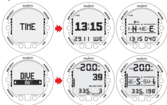
IF ACCESSED FROM TIME MODE, TIME AND BEARING ARE DISPLAYED AT THE BOTTOM OF THE SCREEN.
