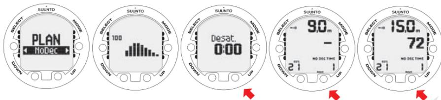
WHEN ENTERING THE MEMPLAN MODE THE DISPLAY FIRST BRIEFLY SHOWS TISSUE LOADING, THE REMAINING DESATURATION TIME BEFORE GOING INTO PLAN MODE. USE UP AND DOWN BUTTONS TO SCROLL DIFFERENT NO-DECOMPRESSION LIMITS. NO-DECOMPRESSION LIMITS LONGER THAN 99 MINUTES ARE DISPLAYED AS "-".
