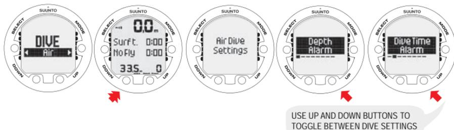
**NOTE** *The settings cannot be activated until 5 minutes has elapsed after the dive.*
