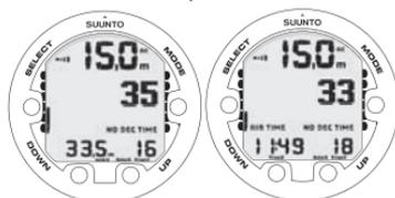
DOWN BUTTON TOGGLES BETWEEN MAXIMUM DEPTH AND CURRENT TIME.
