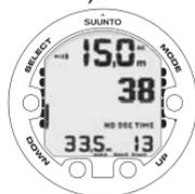
DIVE DISPLAY - PRESENT DEPTH IS 15 M, NO-DECOMPRESSION STOP TIME LIMIT IS 38 MIN. ELAPSED DIVE TIME IS 13 MIN.
