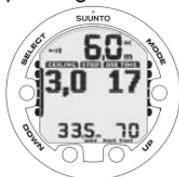
UPWARD POINTING ARROW HAS DISAPPEARED AND ASC TIME LABEL HAS STOPPED BLINKING, MEANING YOU ARE IN THE DECOMPRESSION RANGE.
