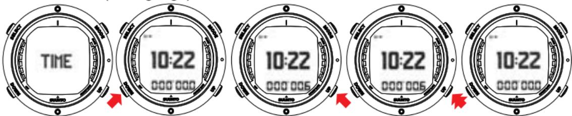
USE DOWN BUTTON TO START STOPWATCH AND TAKE A SPLIT TIME. THE UP BUTTON STOPS THE STOPWATCH AND LONG PRESSING IT RESETS IT.
