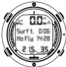
IT IS 6 MINUTES SINCE YOU SURFACED FROM A 35-MINUTE DIVE. THE MAXIMUM DEPTH WAS 21.5 M. THE PRESENT DEPTH IS 0.0 M. THE AIRPLANE SYMBOL AND NO-FLY VALUE INDICATE THAT YOU SHOULD NOT FLY FOR 14 HOURS, 28 MINUTES. THE DIVER ATTENTION SYMBOL INDICATES THAT YOU SHOULD PROLONG YOUR SURFACE INTERVAL TIME.
