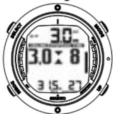
TWO ARROWS POINT AT EACH OTHER “HOUR GLASS”: YOU ARE IN THE OPTIMUM CEILING ZONE AT 3 M. AND YOUR MINIMUM ASCENT TIME IS 8 MINUTES.
