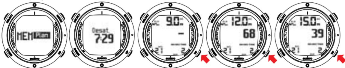
WHEN ENTERING THE MEMPLAN MODE THE DISPLAY FIRST BRIEFLY SHOWS THE REMAINING DESATURATION TIME BEFORE GOING INTO PLAN MODE. USE UP AND DOWN BUTTONS TO SCROLL DIFFERENT NO-DECOMPRESSION LIMITS. NO-DECOMPRESSION LIMITS LONGER THAN 99 MINUTES ARE DISPLAYED AS “—”.
