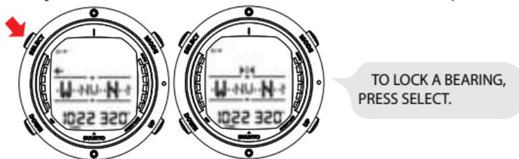
The Suunto D6 also provides help for navigating square and triangular patterns, as well as navigating a return heading. This is made possible by following graphical symbols in the center of the compass display:
