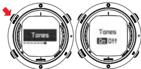
ADJUST WITH UP AND DOWN BUTTONS. ACCEPT WITH SELECT BUTTON.
