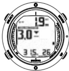
WHEN CEILING AND STOP ARE DISPLAYED, IMMEDIATELY (WITHIN 3 MINUTES) DESCEND TO OR BELOW CEILING.
