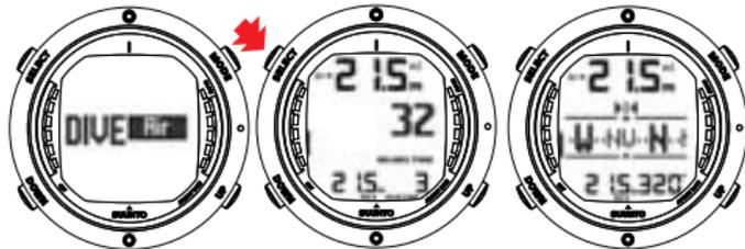
IF ACCESSED FROM DIVE MODE, CURRENT DEPTH AND TIME OR MAXIMUM DEPTH, AS WELL AS BEARING OR DIVE TIME OR TEMPERATURE ARE DISPLAYED.
