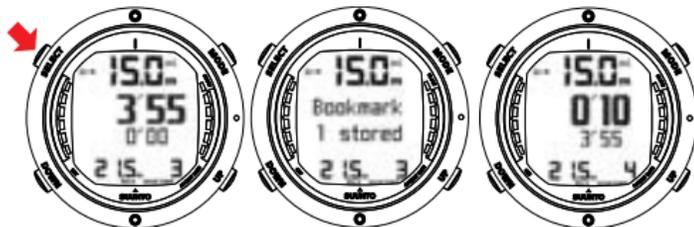
BY PRESSING THE SELECT BUTTON DURING A DIVE, A BOOKMARK IS WRITTEN IN THE PROFILE MEMORY, THE DIVE TIMER IS RESET, AND THE PREVIOUSLY-TIMED INTERVAL IS DISPLAYED BELOW.
