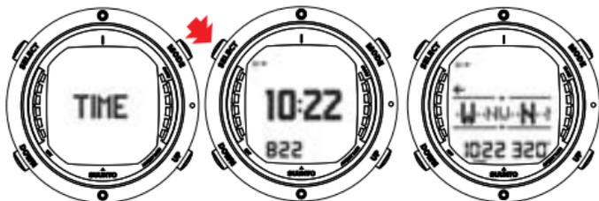
IF ACCESSED FROM TIME MODE, TIME AND BEARING ARE DISPLAYED AT THE BOTTOM OF THE SCREEN.
