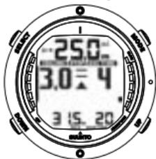
UPWARD POINTING ARROW, BLINKING ASC TIME AND AN ALARM TELL YOU TO ASCEND. MINIMUM TOTAL ASCENT TIME INCLUDING SAFETY STOP IS 4 MINUTES. CEILING IS AT 3 M.
