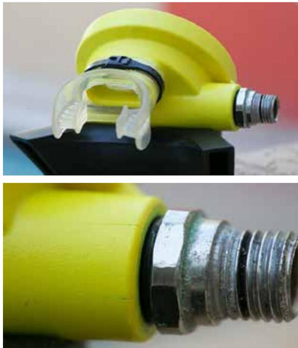
Figure 3-5. Plastic second-stage regulators with microfractures
